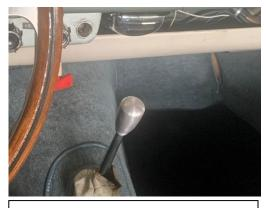
aluminium gear lever knob made for TD21
